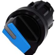
Selector switch, illuminable, 22 mm, round, plastic, blue, selector switch, short, 2 switch positions O<I, momentary contact type, Actuating angle 45°, 10:30h/12h, with laser labeling, upper case and lower case, always upper case at the beginning of the word
