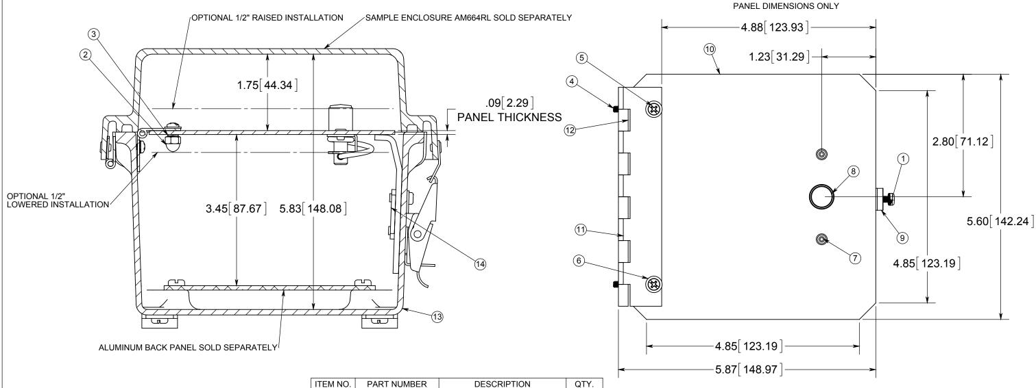
NOT ALL PARTS OF THE HFP ASSEMBLY KIT ARE SHOWN, ONLY THE PARTS USED IN THE FLUSH INSTALLATION OF THE PANEL. FOLLOW INSTALLATION INSTRUCTIONS INCLUDED IN THE KIT FOR THE OPTIONAL PANEL MOUNTING.
