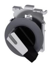
Selector switch, illuminable, 30 mm, round, Metal, matte, white, selector switch, long, front ring for flush installation, 2 switch positions O-I, latching, actuating angle  $90^{\circ}$ , 10:30h/13:30h, with laser labeling, upper case
