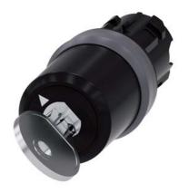
Key-operated switch BKS, 22 mm, round, plastic with metal front ring, Lock No. E7 (VW), without key, 2 switch positions O-I, latching, actuating angle  $90^{\circ}$ , 10:30h/13:30h, key removal O, with laser labeling, upper case and lower case, always upper case at the beginning of the word
