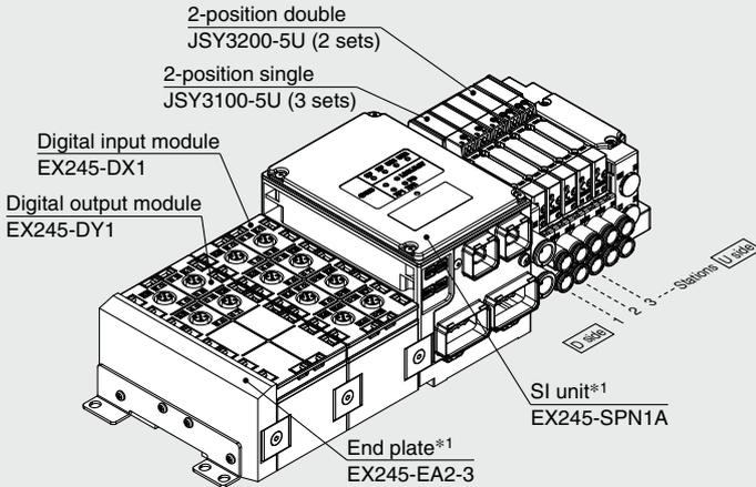
JJ5SY3-10SAANY2-05D-C6... 1 set (Type 10 5-station manifold base part no.)
