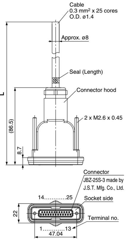
**D-sub connector cable [IP20/40 compliant]**
