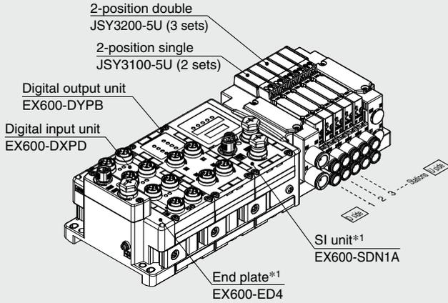
JJ5SY3-10S6Q72-05D-C8 .. 1 set (Type 10 5-station manifold base part no.)
