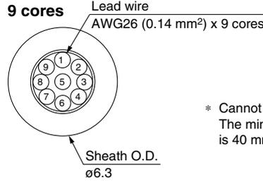
\* Cannot be used for movable wiring
