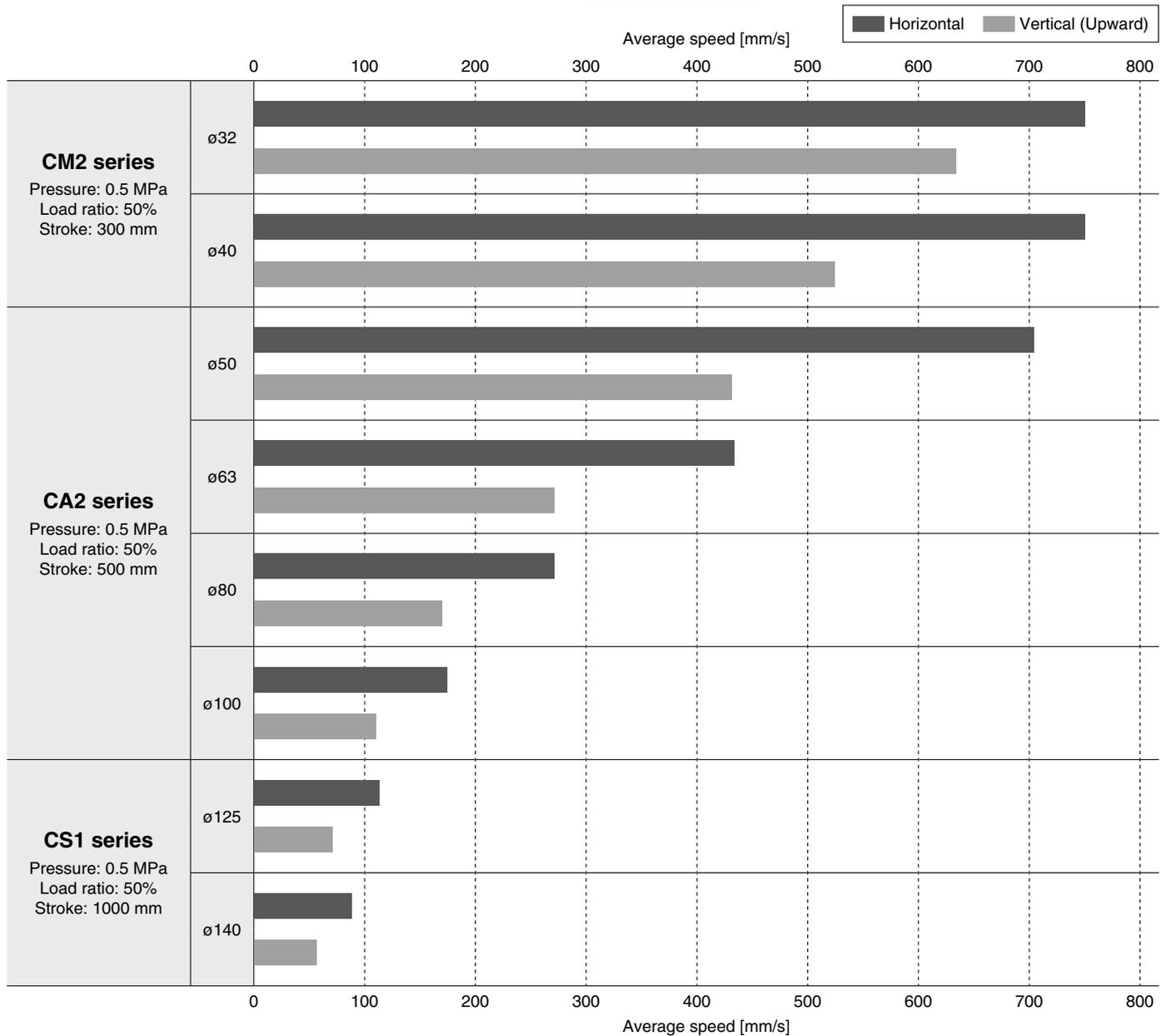
\* Values at extension of a directly coupled cylinder when meter-out speed controllers are used with the needle full open.
