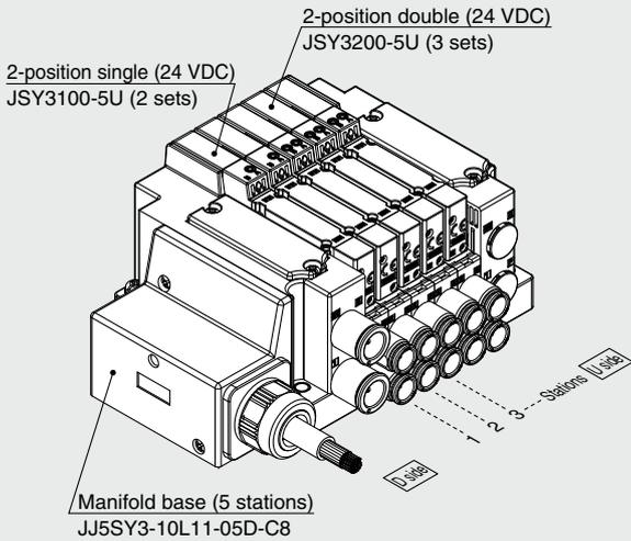
**JJ5SY3-10L11-05D-C8** 1 set (Type 10 5-station manifold base part no.)
