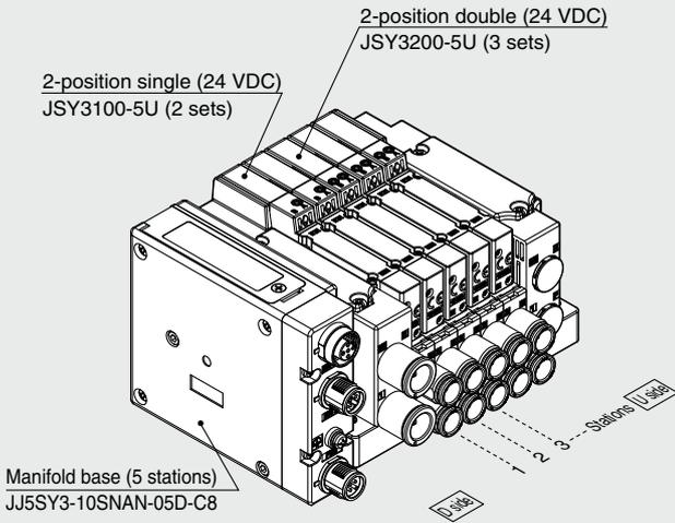
**JJ5SY3-10SNAN-05D-C8** .. 1 set (Type 10 5-station manifold base part no.)
