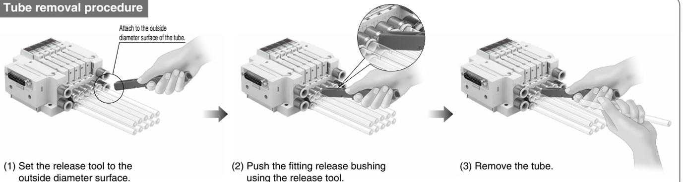
(1) Set the release tool to the outside diameter surface.
