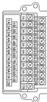
If alignment is not specified, the internal wiring will be double wiring (connected to SOL. a and SOL. b) regardless of number of stations, valve types, and option types.
