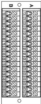
If alignment is not specified, the internal wiring will be double wiring (connected to SOL. a and SOL. b) regardless of number of stations, valve types, and option types.
