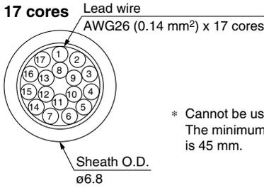
\* Cannot be used for movable wiring
