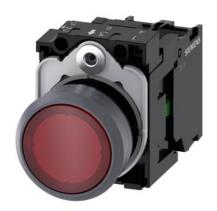
Illuminated pushbutton, 22 mm, round, plastic with metal front ring, red, pushbutton, flat, momentary contact type, with holder, 1NO, LED module with integrated LED 24 V AC/DC, screw terminal, with laser labeling, upper case
