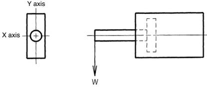
\* In case of a plate cylinder, although there is the case that a load is applied in both X and Y axis as illustrated, but the allowable lateral load is the same.
