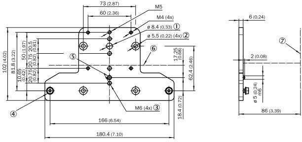
① Rotation point for cylinder pin ø 8.2 mm (part 2079939)
