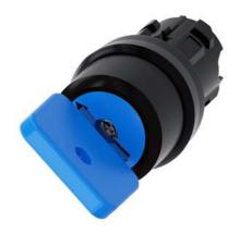
Key-operated switch O.M.R, 22 mm, round, plastic, lock number 73038, blue, with 2 keys, 2 switch positions O-I, latching, actuating angle 90°, 10:30h/13:30h, key removal O+I, with laser labeling, upper case and lower case, always upper case at the beginning of the word
