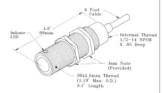
Quick Disconnect fitting adds .35" (9 mm) in overall length to QD models. QD models require Quick Disconnect cable (order separately; see Specifications section for information).
