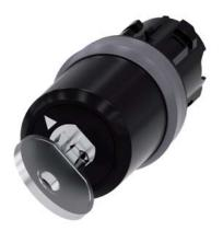
key-operated switch Siemens, 22 mm, round, plastic with metal front ring, lock number SSG10, with 2 keys, 2 switch positions O<I, momentary contact type, actuating angle  $45^\circ, 10:\!30h/12h,$  key removal O, with laser labeling, upper case and lower case, always upper case at beginning of line
