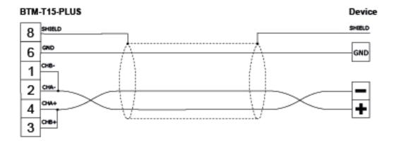
Fig. 9 Connection diagram for RS485\*\*
