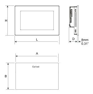
Fig. 2 Dimensions BTM-T15-PLUS
