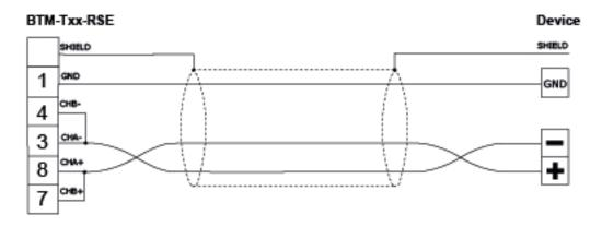
Fig. 8 Connection diagram for RS485\*\*
