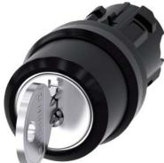
RONIS key-operated switch, 22 mm, round, plastic, lock number SB30, with 2 keys, 3 switch positions I>O<II, momentary contact type, actuating angle 2x45°, 10:30h/12h/13:30h, key removal O, possible special locks: SB31, 421, 455 Z=50-unit packaging
