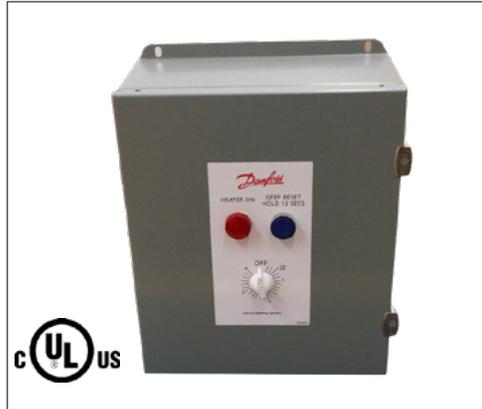
The Danfoss GFEP Contactor Panel is primarily designed for snow and ice melting applications. The integral 30mA Ground Fault Protection Equipment (GFEP) ensures safety along with NEC and local codes requirements. The panel can be activated by a Danfoss GX850, DS-2C, DS-5C, DS-8C or other type of controller.
