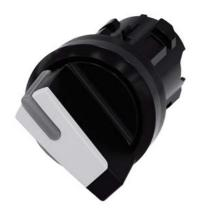
Selector switch, illuminable, 22 mm, round, plastic, white, selector switch, short, 2 switch positions O-I, latching, actuating angle  $90^\circ,\,10:\!30h/13:\!30h$
