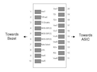
Pin-out of connector Block on Host board
