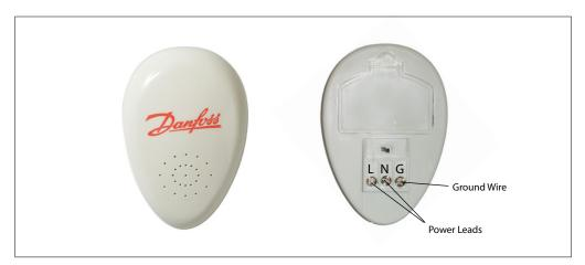
Simplify your installation process using the Little Buzzer by Danfoss! The Little Buzzer is designed to monitor Danfoss heating mats and/or cables during the installation process and sounds an alarm if the heating elements are cut or damaged. This allows easy repair before the floor coverings are laid. The device is battery powered (batteries included).
