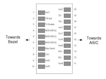
Pin-out of connector Block on Host board
