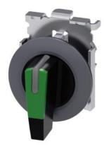
Selector switch, illuminable, 30 mm, round, Metal, matte, green, selector switch, long, front ring for flush installation, 3 switch positions I>O<II, momentary contact type, actuating angle 2x45°, 10:30h/12h/13:30h, with laser labeling, inscription or symbol Customer-specific selection with SIRIUS ACT configurator (CIN)
