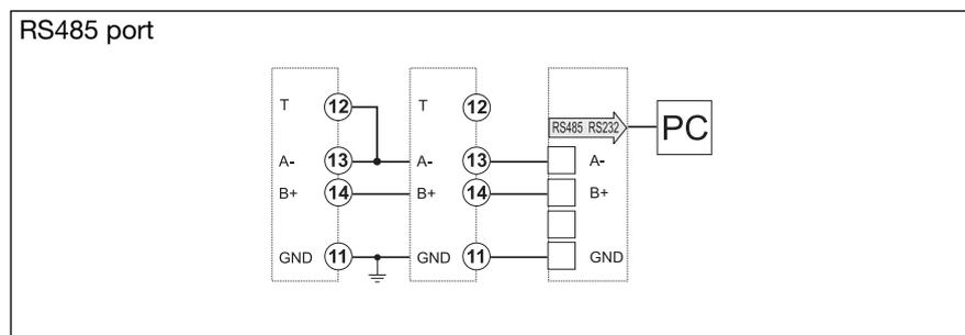
**RS485 NOTE:** additional devices provided with RS485 are connected in parallel. The termination of the serial output is carried out only on the last instrument of the network, by means of a jumper between (A-) and (T).
