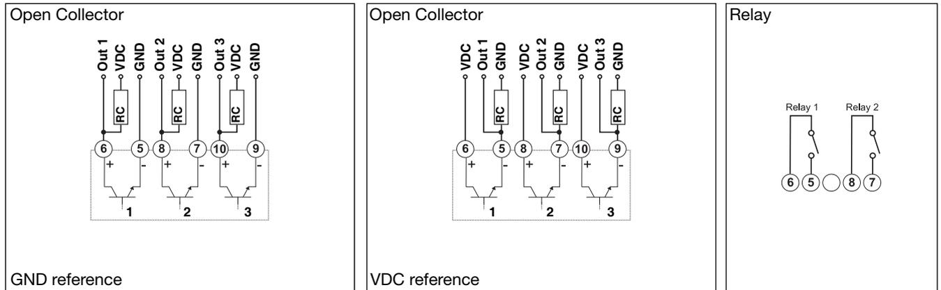
The load resistances (RC) must be designed so that the close contact current is lower than 100mA; the VDC voltage must be lower than or equal to 30VDC.
