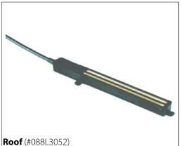
The Danfoss digital sensors are used with the GX 850 Automatic Control Panel and the GX 850M Controller - the most optimal solutions for keeping an area free of ice and snow. The controllers act on information received from the sensor(s), which register both temperature and moisture, and then calculates the information ensuring that the heat will only be turned on when snow and/or ice is present. The result is optimal performance with maximum energy savings and minimum operating costs.
