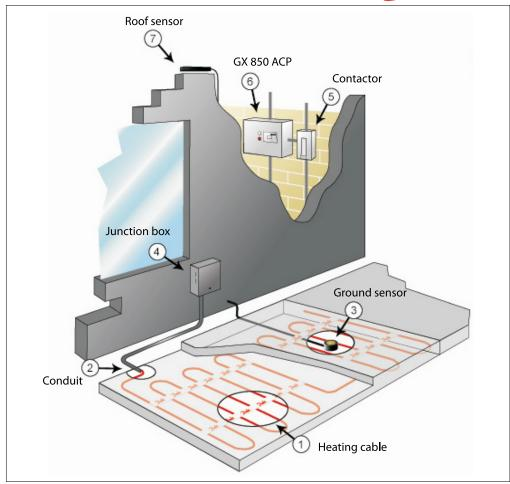
Note: Danfoss recommends a minimum of two ground sensors per heating zone.
