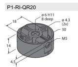
1593041 Positioning element for encoder RI-QR20, for Ø 6 mm shafts
