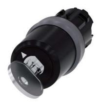
Key-operated switch BKS, 22 mm, round, plastic with metal front ring, lock number S1, with 2 keys, 2 switch positions O-I, latching, actuating angle  $90^\circ, 10:\!30h/13:\!30h,$  key removal O, with laser labeling, upper case
