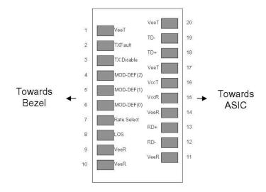
Pin-out of connector Block on Host board
