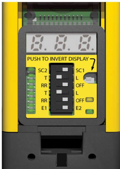
Figure 24. EZ-SCREEN Configuration DIP Switches (Receiver)
