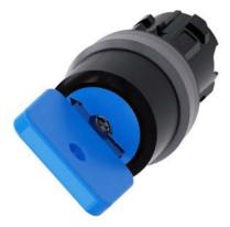
Key-operated switch O.M.R, 22 mm, round, plastic with metal front ring, lock number 73038, blue, with 2 keys, 2 switch positions O<I, momentary contact type, Actuating angle 45°, 10:30h/12h, key removal O, with laser labeling, upper case and lower case, always upper case at beginning of line
