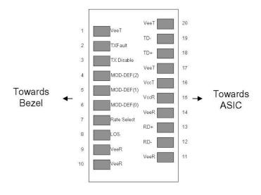
Pin-out of connector Block on Host board
