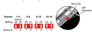
By default, the LMRH-105 controls DLM scenes 1-4. Users can select a different group of four scenes by resetting DIP switches located in the battery compartment.
