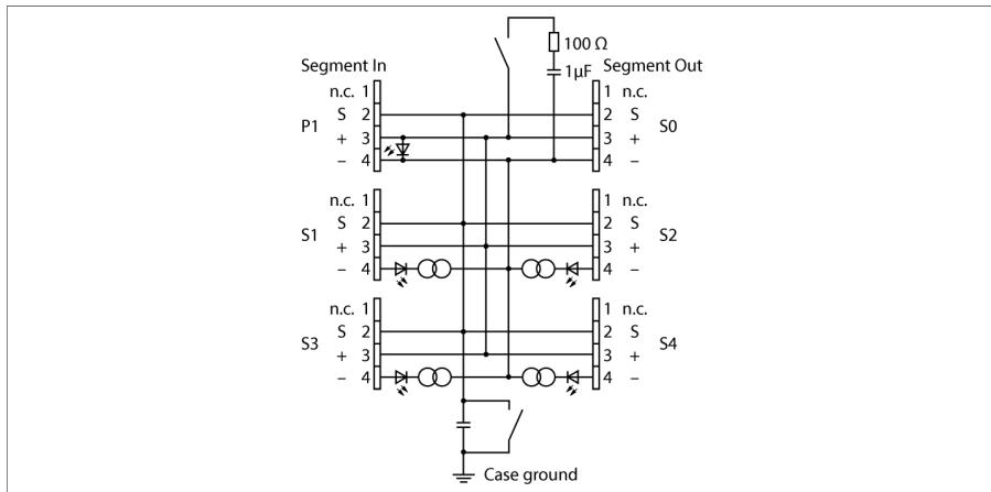
The 4-channel Ex junction box JBBS-49SC-T415B/EX is designed for FOUNDATION™ fieldbus systems.
