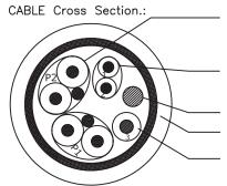
Conductor:2P\*30AWG(7/0.10 Tinned Copper) Isulation: %0.79 (LDPE)
